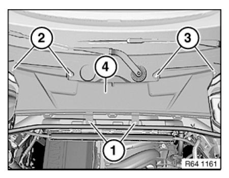
Release screws (1). Unfasten screws (2 and 3). Remove upper section of microfilter housing (4).
