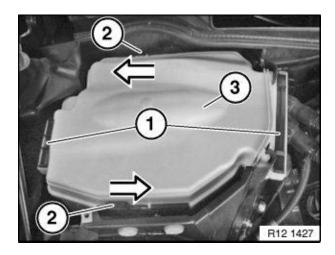
Unlock fasteners (1) from below and slide upwards approx. 10 mm.
