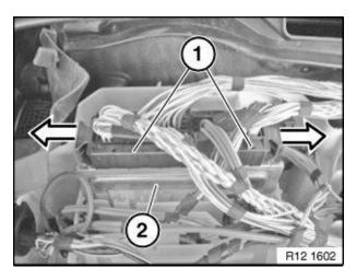
Unlock connectors (1) using slide in direction of arrow and remove.
