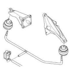
The default position is the "hard" setting when no vacuum is present at the engine mounts.
