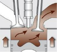
Exhaust Stroke Diesel Engine
