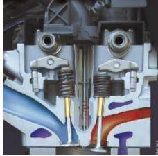
Cylinder head cross section **Diesel Engine**
