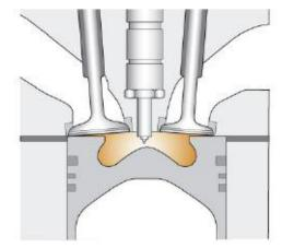
For example, the shape of the combustion chamber has an effect on fuel mixing. The mixture can be influenced or "shaped' by the piston design and the angle at which the fuel is injected. The intake manifold and intake ports can be designed to provide more air motion in the combustion chamber. This is referred to as the "swirl effect". By providing this air movement via "swirl", the air is better mixed with the atomized fuel and thus contributes to lowered emissions.
