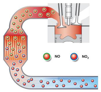
One of the major factors in the formation of  $NO_X$  is the overall combustion chamber temperature. Diesel engines have inherent issues regarding the production of  $NO_X$ .
