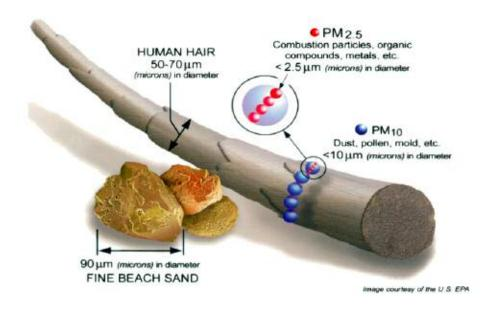
Diesel exhaust consists of mostly the smaller (PM2.5) particles. Particulate matter is considered a harmful pollutant which contributes to respiratory problems. Therefore, PM emission should be controlled. PM emissions can be reduced in a number of ways. One of the first and most practical measures is to reduce the sulfur content in the fuel. As of 2007, the new ULSD fuel has a limit of 15 ppm sulfur. This represents a major reduction over the former 500 ppm limit.
