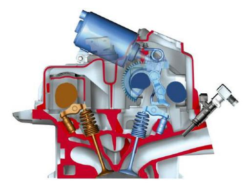
Some of the other engine innovations include high-precision direct fuel injection for gasoline engines. The HPI system allows the N54 engine to maintain maximum performance and astounding fuel economy in a 300 hp engine. To complement all of the engine technology currently in use, BMW will be adding diesel powered BMW's to the model line by the end of 2008. Besides the obvious fuel saving advantages of diesel engines, there are many performance related aspects of this new technology.
