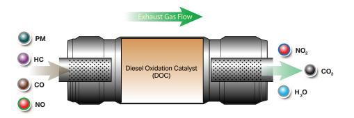
Soot particles flow through the oxidation catalytic converter unimpeded. The oxidation catalytic converter is additionally used to increase the temperature during regeneration of the diesel particulate filter. The ceramic carrier (cordierite) features a platinum-based oxidation coating.
