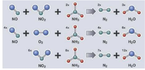
NO<sub>X</sub> reduction: Nitrogen oxides react with ammonia to form nitrogen and water
