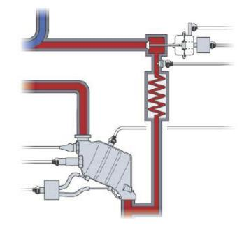
The following graphic shows the control of the EGR system with low pressure EGR:
