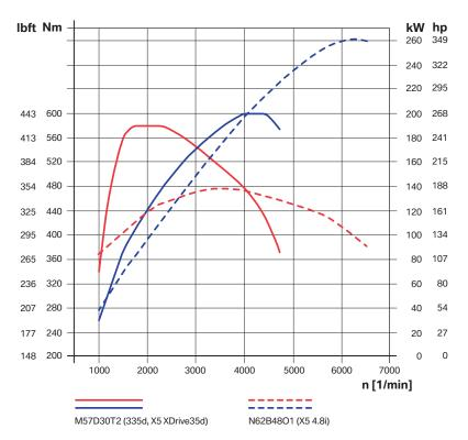
The familiar N62B48O1 has impressive horsepower output but, even with 8-cylinders, it does not have the torque output of the M57 diesel engine.
