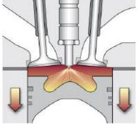
Power Stroke Diesel Engine
