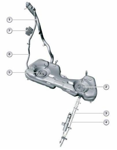
As with current gasoline fuel injection systems, there is an electric fuel pump located in the fuel tank. The fuel pump supplies the needed low pressure fuel to feed the mechanical high-pressure pump.
