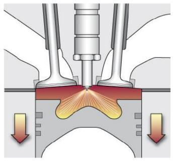
The injection system on a diesel engine functions, in some ways, much like an ignition system on a gasoline engine. In order to start combustion, it is necessary to inject fuel at the right time with reference to the position of the piston. Just like an ignition system on a gasoline engine, the injector must inject fuel before top dead center (BTDC).
