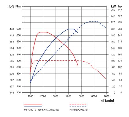
The following full load diagrams provide a comparison of the new diesel engine to the current production gasoline engines, both 6 and 8 cylinder.
