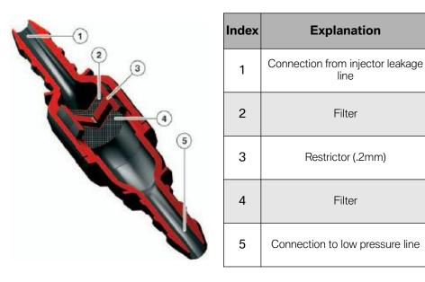
The fuel flowing from the piezo-fuel injectors via the fuel return connection (1) initially passes through a filter (2), through restrictor (3) and then through a further filter (4) to connection (5) back into the fuel feed to the high pressure pump.
