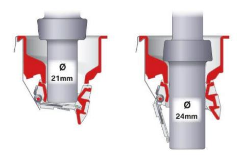
As the following illustrations show, only a fuel nozzle with a diameter of approximately 24 mm can fit. If the diameter is approximately 21 mm, the flap (4) does not open as the hinged lever (7) and the locking lever (2) cannot be pushed apart.
