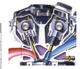
Cylinder head cross section Gasoline Engine
